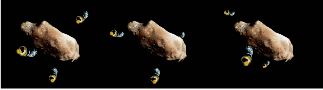
Figure 1. Concept illustration of multiple satellite spacecraft in orbit around an asteroid. Left: all three have line-of-sight and may communicate point-to-point. Middle: each has different orbitals, one spacecraft is behind the asteroid and its line-of-sight is occluded. Right: a later time-frame snapshot showing reestablished line-of-sight and different positional coordinates. (The Galileo spacecraft shown here replicated three times photographed Asteroid 243 Ida also shown in this picture, during its fly-by on August 28, 1993; images by courtesy of NASA and NASA/JPL-Caltech).
